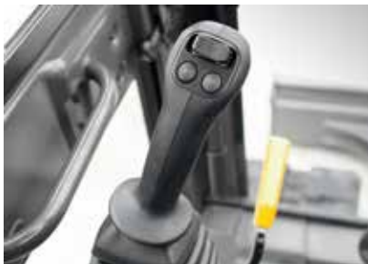
Electric dozer blade switch on joystick
