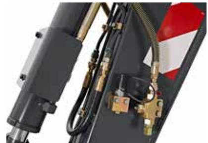
Auxiliary hydraulic piping (X3)
