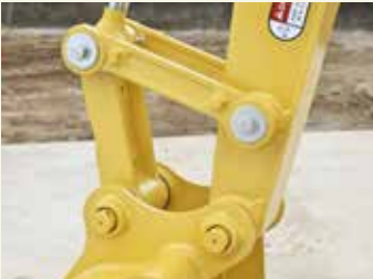
Bucket Cast-iron idler links provide greater strength.
