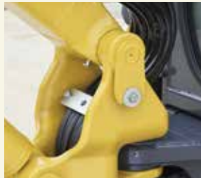
Hydraulic piping The hydraulic piping is housed inside the swing bracket for protection.
