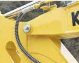
Bolt-tightened pins firmly lock the boom and arm for increased durability.
