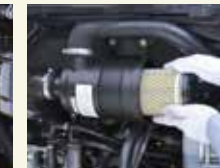
Pre fuel filter with built-in water separator
