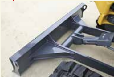
Dozer Box construction dozer supports provide greater strength.
