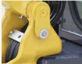
Plate type pin head prevent wear by rotation of the pin itself. Thick swing bracket.
